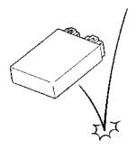
Be careful not to touch the electrical terminals of the electronic parts (ECM, etc.). The static electricity from your body may damage these.
