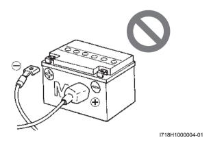
Removing any battery terminal of a running engine is strictly prohibited. The moment such removal is made, damaging counter electromotive force will be applied to the ECM which may result in serious damage.
