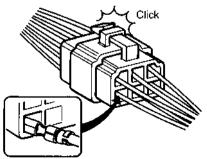
Inspect each lead wire circuit for poor connection by shaking it by hand lightly. If any abnormal condition is found, repair or replace.
