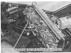
(4) The throttle body identification number is stamped on the intake side of the throttle body as shown.
