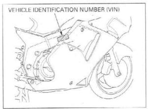
(3) The Vehicle Identification Number (VIN) is located on right side of the frame near the steering head on the Safety Certification Label.
